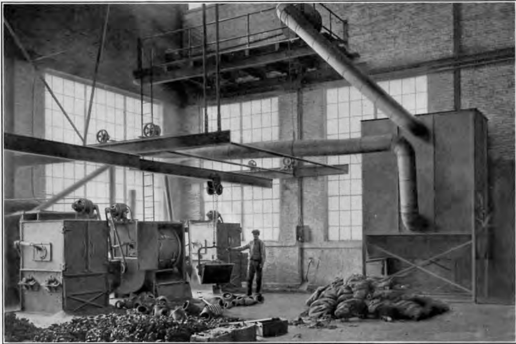
Battery of Three Pressure Type Barrels Cleaning Malleable Fittings. Castings brought and removed by mono-rail buckets. American Cloth Screen Dust Arrester No. 6 at the right.
