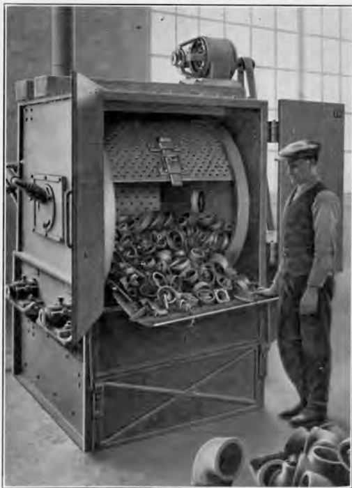
Pressure Barrel Open, Showing Finished Castings Ready for Removal. Individual motor drive can be supplied if especially ordered.
